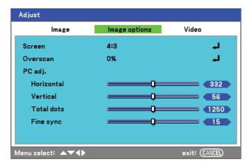
5. Select the desired picture size using ▲ or ▼ and press ←.
